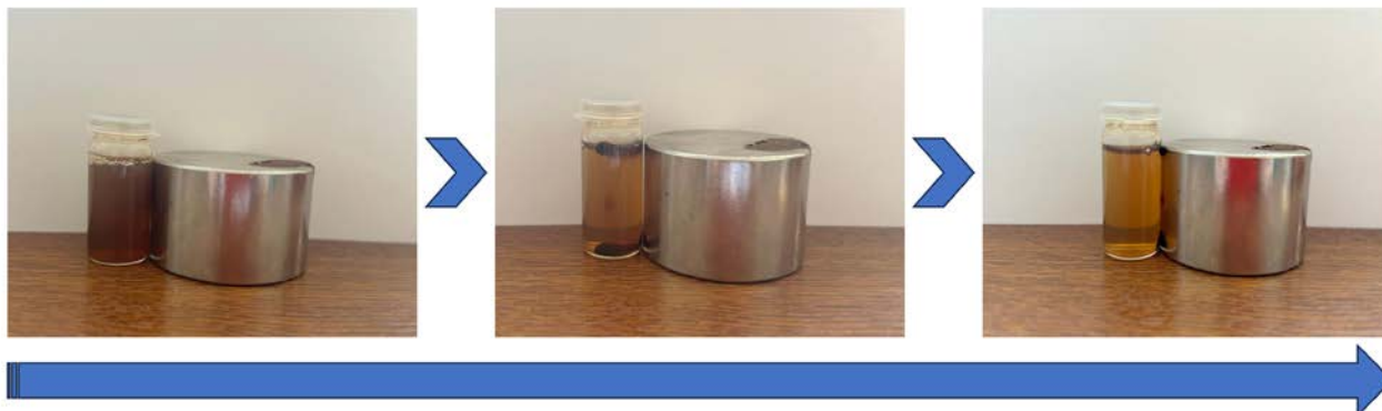
MLL0.5 nanoparticles migration towards permanent magnet over time
